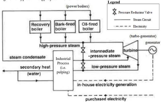
Figure 2: Typical Energy System for a Kraft Mill<sup>5</sup>
