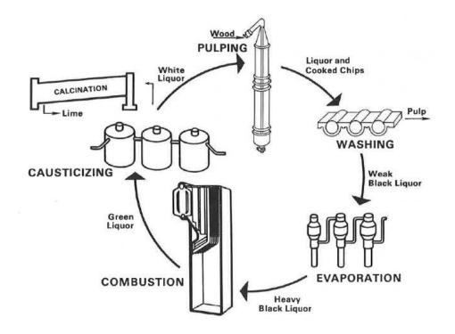
Figure 1: Schematic diagram of Kraft Pulping and Chemical Recovery Cycle<sup>4</sup>
