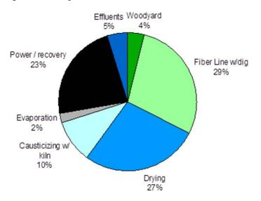
Figure 4: Example Kraft Mill Maintenance Allocation
