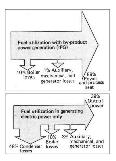
Figure 3: Generation Comparison of Backpressure (Top) and Condensing (Bottom)  $\mathsf{Power}^6$
