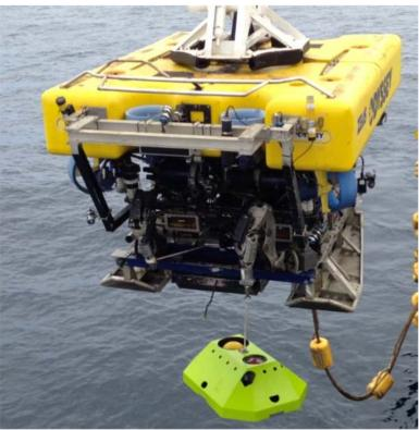
**ROV being lowered into the water with equipment to test water column currents and turbidity** (to assist with the plume dispersion model)
