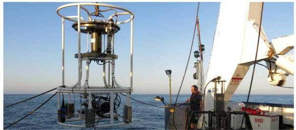
**Carousel Water Sampler being lowered into the water column structure across the Project area** (*temperature, salinity, turbidity, light penetration*)
