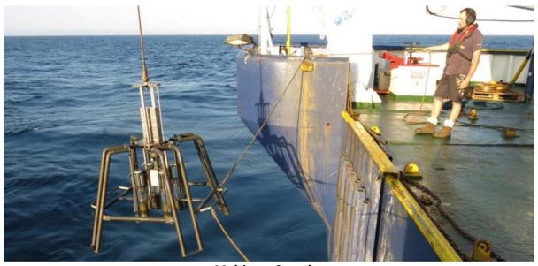
**Multicore Sampler** (used to characterize ore and overburden at site for input into plume modelling and dredging locations)
